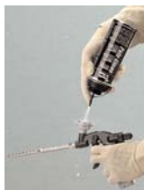
Spray cleaner directly on top of gun for foam removal.
